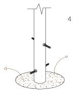
Excavate 7 holes with a 250mm diameter tapering down to 350mm diameter
