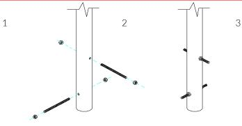
Insert M10x 200 Threaded bar into pre drilled holes in **Ground Fixing Post**
