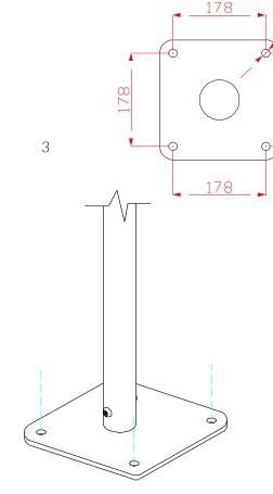
Fix Surface Plate to the ground surface **Ground Anchors Not provided** cover fixings with caps provided
