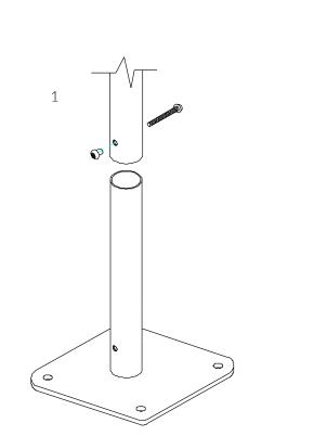
Locate the Surface fix Plate into the leg of the instrument. Fix instrument to Surface fix plate using M10 bolt and Barrel Nut and use **thread locking solution** to prevent fixings working loose.
