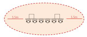
Install Instrument with 1.5m free space (from widest point) around it.
