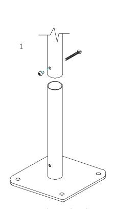
Locate the Surface fix Plate into the leg of the instrument. Fix instrument to Surface fix plate using M10 bolt and Barrel Nut and use **thread locking solution** to prevent fixings working loose.
