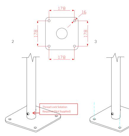
Fix instrument to Surface fix plate using M10 bolt and Barrel Nut and use **thread locking solution** to prevent fixings working loose.
