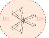
Install Instrument with 1.5m free space (from widest point) around it.
