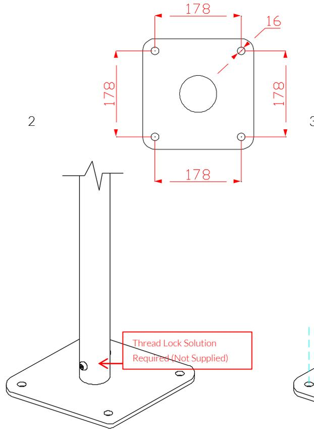
Fix instrument to Surface fix plate using M10 bolt and Barrel Nut and use **thread locking solution** to prevent fixings working loose.
