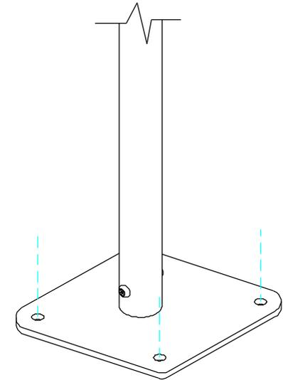
Fix Surface Plate to the ground surface **Ground Anchors Not provided** cover fixings with caps provided
