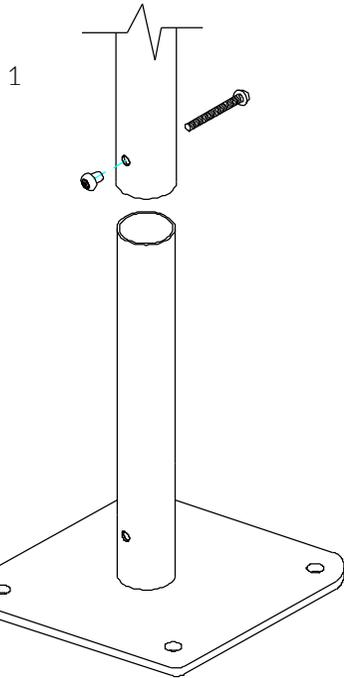
Locate the Surface fix Plate into the leg of the instrument.
