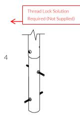
Fix instrument to Ground fix post using M10 bolt and Barrel Nut and use thread locking solution to prevent fixings working loose.
