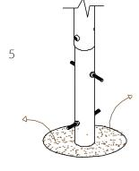
Excavate 1 hole with a 250mm diameter tapering down to 350mm diameter and 650mm depth
