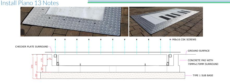
Once happy with piano installed, finally attach the checker plate surrounds with screws provided making sure clearance gaps are even all around the notes. Use Square washers to adjust height of tread plate according to surface levels.
